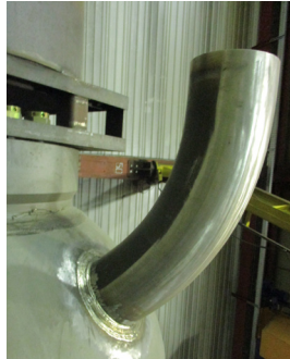
Elbow by seamless tube, bent and welded on hemispheric head
