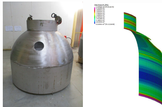
Forming by hydraulic pressure, design by finite element analysis
