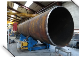
~ 80mm tickness + Protective Layer by Lining
