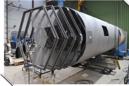
Clamped Baffle Support with Low Flow Resistivity
